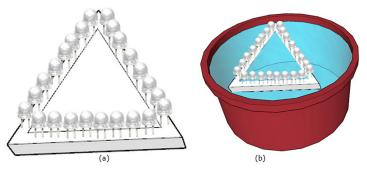
Figure 4. 24-LED triangle configuration: (a) positioning of the LEDs and (b) location above the water
