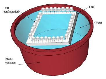
Figure 7. Light trap with LEDs at 1 cm from the water
