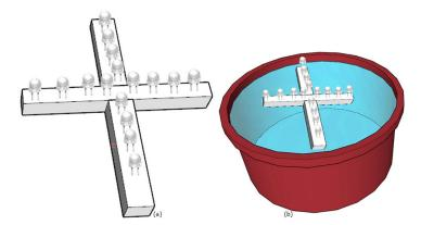
Figure 5. 16-LED cross configuration: (a) positioning of the LEDs and b) location on the water
